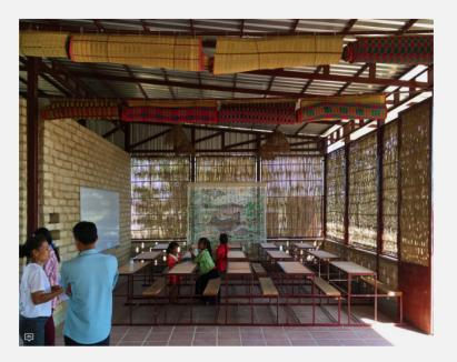
The masterplan elements are designed to be responsive to the tropical climate – with raised floors to negate flood risk, screens to diffuse sunlight whilst providing ventilation, and overhanging roof eaves for the rainy season – as well as utilising local resources, labour and skills.
