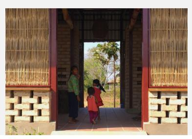
The main structure provides a multi-use hall with office and storage spaces, and a full width screened veranda. Within a robust rectangular steel frame, the primary building materials comprise bricks made on site from stabilised earth, rice husk/clay blocks and bamboo screens. Cassava and sand plaster is used to render walls, created in collaboration with local organic farm OrganiKH.
